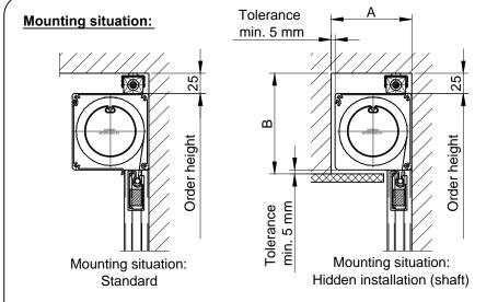
Dimensions shaft (in case of hidden installation + guide rail 30x30 mm):
